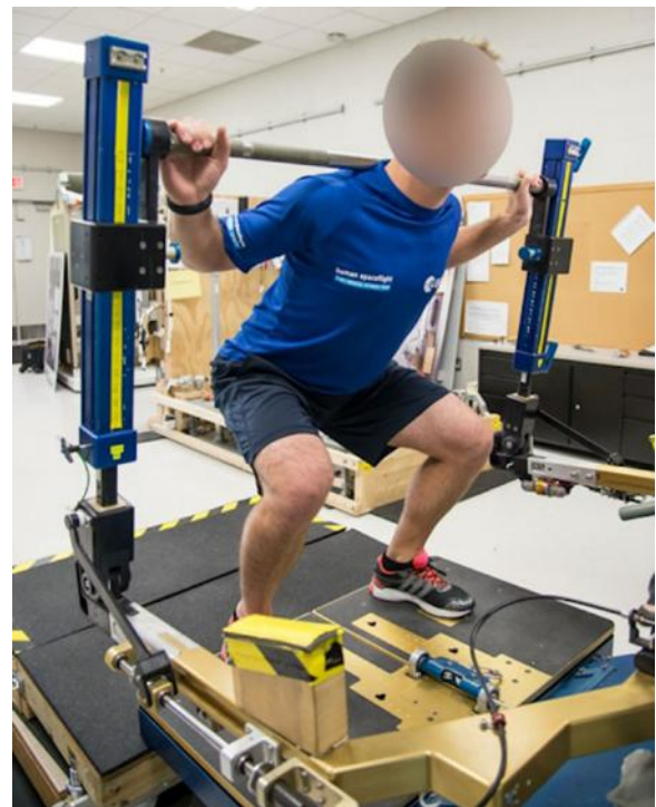
Fig. 2. Familiarization with the Advanced Resistive Exercise Device (ARED) on Earth before spaceflight (squatting). These sessions focus on optimizing spinal posture during exercise. Photo credit: © ESA/NASA.
